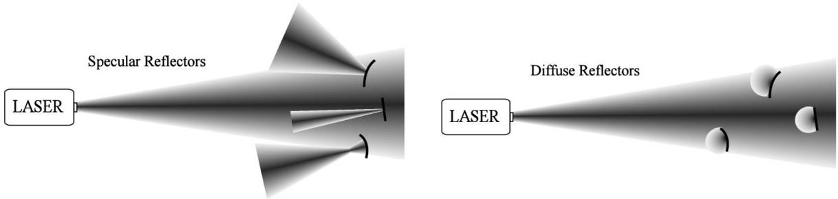
**Figure 2-3. Effects of Specular Reflector and Diffuse Reflector on Incident Laser Beam**
