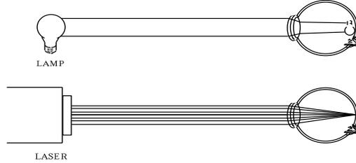
**Figure 2-5. Focusing of Laser Beam and Conventional Light Source by the Eye**
