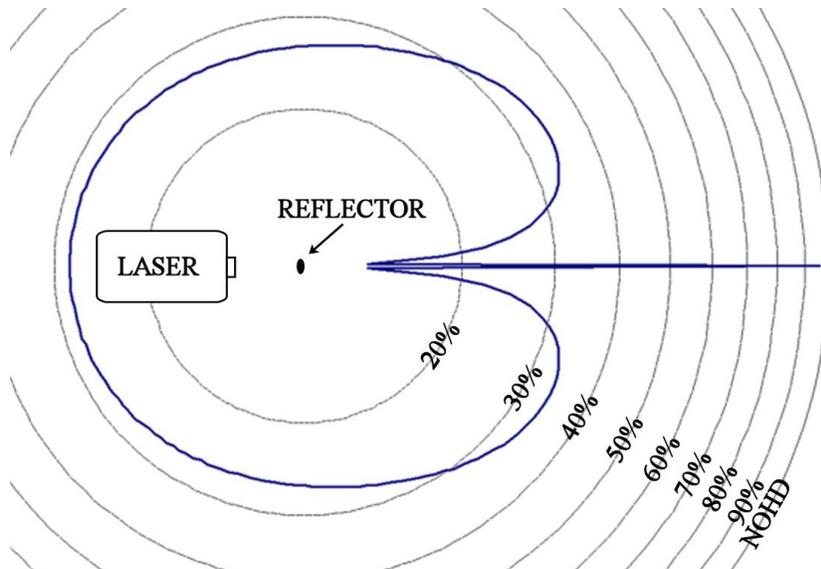
**Figure 2-4. Hazard Zone Created by Reflected Laser Energy from a Randomly Oriented Circular Piece of Glass**
