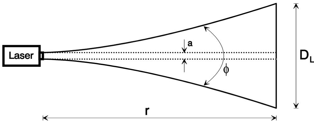
Figure 2-1. Laser Beam Geometry
